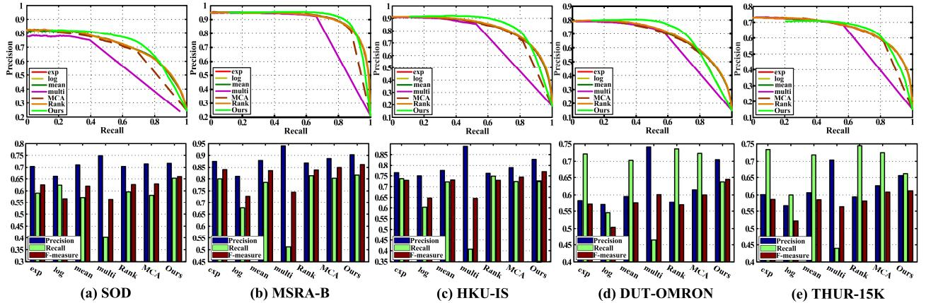
Fig. 10. Performance comparisons of the proposed approach and other fusion based saliency detection approaches [2], [27], and [35] in terms of PR-curves, Precision, Recall and F-measure on the SOD, MSRA-B, HKU-IS, DUT-OMRON, and THUR-15K datasets.
