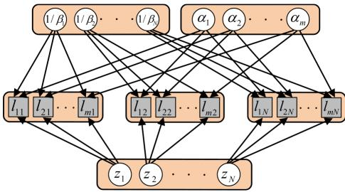
Fig. 3. Graphic model of each superpixel's labeling difficulty, each weak saliency label's labeling accuracy, the superpixel's weak saliency labels, and real saliency label. Only the shaded variables are available during the inference process.
