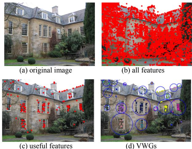
Figure2. For an input image (a), we extract 4002 raw SIFT points which are shown in (b). (c) shows the selected 169 useful visual words. In (d), we generate 24 visual word groups.
