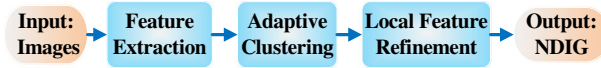
Fig. 2 Block diagram of near duplicate image groups mining. A system contains adaptive clustering to find out the potential near duplicate image groups, and local feature refinement to make sure the selected groups are true near duplicates
