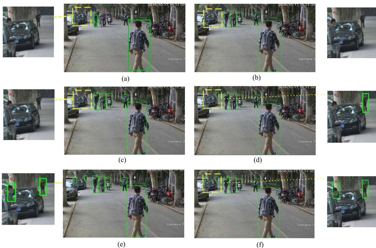
**FIGURE 10.** The comparison of four methods in XJTU Pedestrian dataset for pedestrian detection. (a) YOLO9000. (b) SSD512. (c) Faster R-CNN. (d) PVANET. (e) MPNET(Faster R-CNN). (f) MPNET(PVANET).
