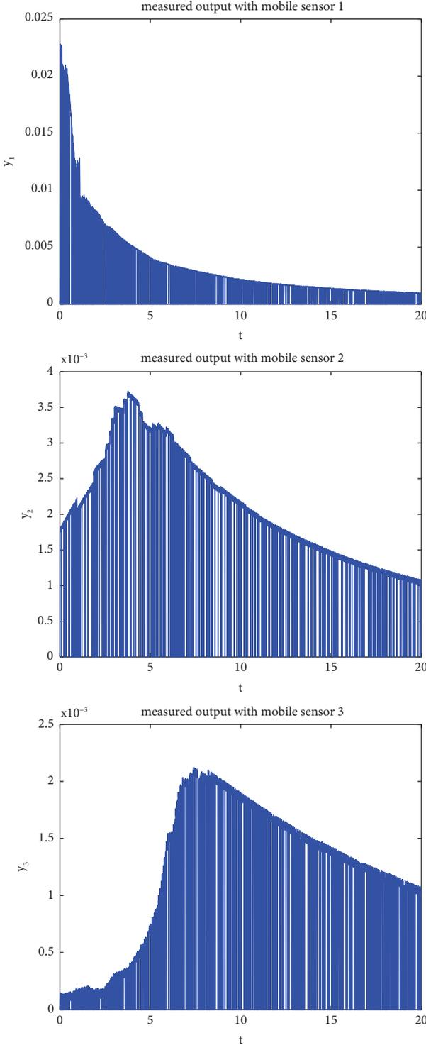
FIGURE 2: The output of moving sensors with random missing data.
